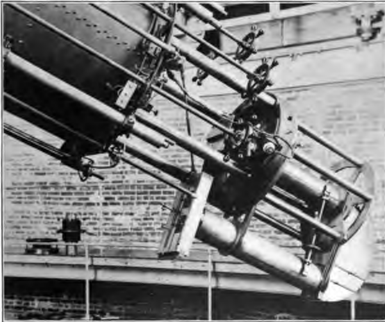
FIG. 2.—Spectroheliograph attached to 40-inch Yerkes Refractor.
